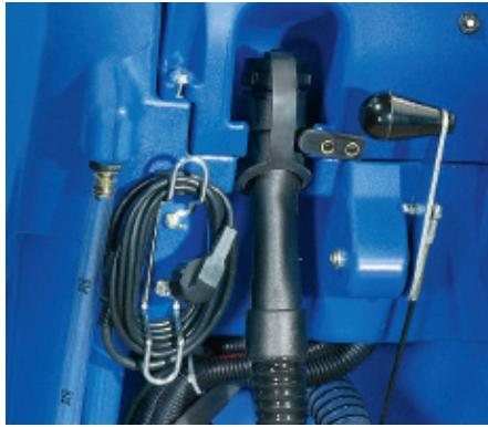
Rear solution fill allows filling when the machine is back into the deep sink for emptying the recovery
