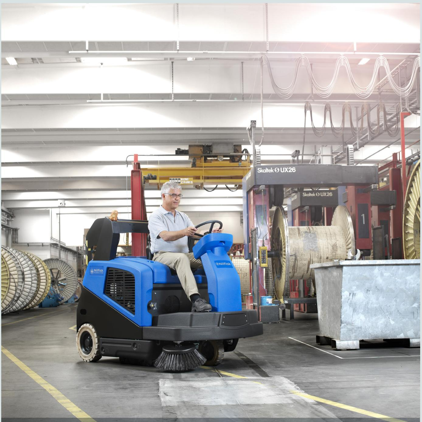
From the driving position, you can monitor and fully control all cleaning functions just by pushing a few buttons. The high performance comes down to the one touch sweeping principle of the machine. When not driving sweeping functions stop automatically, saving energy, reducing broom wear and making operation easy.
