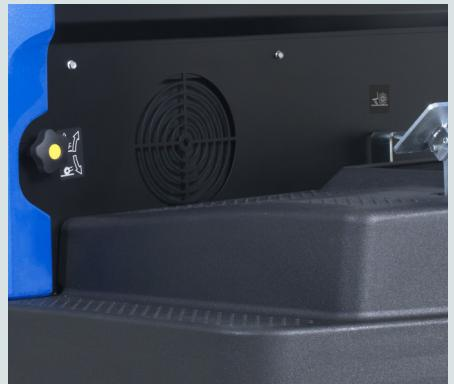
The main broom can be adjusted by one knob reachable from the driver's seat
