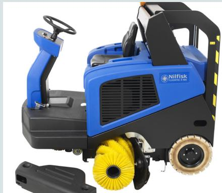
Replace the main broom in less than a minute - without any tools
