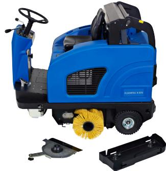
No tools are needed for main or side broom and filter removal and easy access to all components makes for fast and easy maintenance and service.
