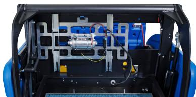
Filter can be changed/inspected on LPG models without removing the LPG bottle, this is therefore more ergonomic and faster.
