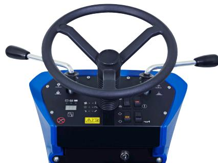
One-touch sweeping control. All functions start automatically when brooms are lowered and the machine is activated. Means less need for operator training.
